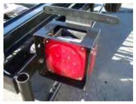
**Rear LED Light Assembly** – Use a **13mm ratchet** or **open end wrench** to attach rear light protectors to the frame as shown below. The tail lights are plug & play, locate the wire harness for the rear lights on the frame and plug in the connector from the lights into the wire harness on the trailer frame as shown below.
