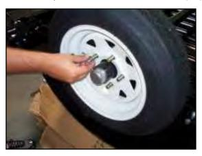
**STEP 11:** Tire/Wheel Assembly – Remove the wheel lug nuts from the hubs, and slide the complete tire/wheel assembly as shown above with valve stems facing outward on the lugs of each hub. **Use the 22mm ratchet with extension** to properly secure lug nuts back onto the wheel with 65-70 ft-lb torque.
