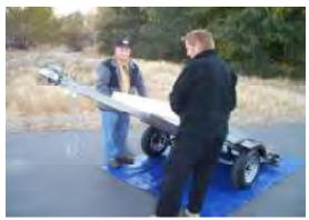
**STEP 13; USE EXTREME CAUTION:** Using at least (2) strong bodied people, safely flip the trailer over by standing the trailer on end (its rear frame) and carefully flipping it over to support itself on the wheels and the tongue stand. **Do not attempt this if you do not have;** 1.) Adequate clearance above and from side to side or 2.) Enough man power that can SAFELY handle the weight of the trailer when flipping it over.
