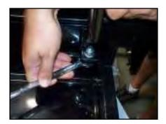
**STEP 6:** Use the **19mm ratchet & open end wrench** to attach and securely tighten the (4) 1" long bolts, washers and lock nuts that fasten the tongue mount to the front of the trailer frame.
