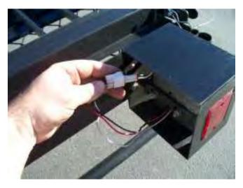
**LED Side Markers** - Use a **small Phillips screw driver** and a **7mm ratchet or open end wrench** to attach side markers to the frame as shown below. Please review the pictures below to make sure the side markers are mounted as shown. The side markers are plug & play. Locate the wire harness for the side markers on the frame and plug in the connectors from the lights into the harness.
