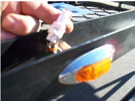
SIDE MARKERS ARE INSTALLED
