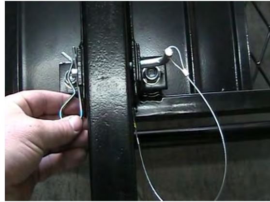
ATTACH PIVOT BOLT & L PIN TO FRAME
